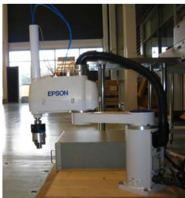
A 4-axis pick-and-place robot has been purchased for use on Wombat and Echidna. A tray containing up to 50 samples is located on a trolley near the robot. This remotely controlled robot then takes
