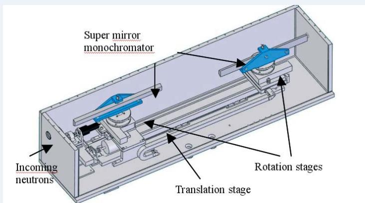
Figure 1. Drawing of the monochromator
