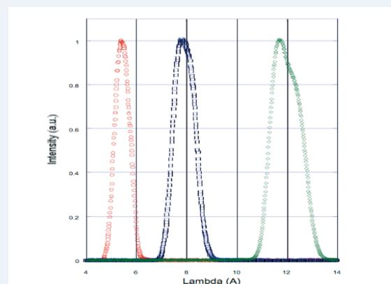
Figure 2. Raw TOF measurements of monochromated beams
