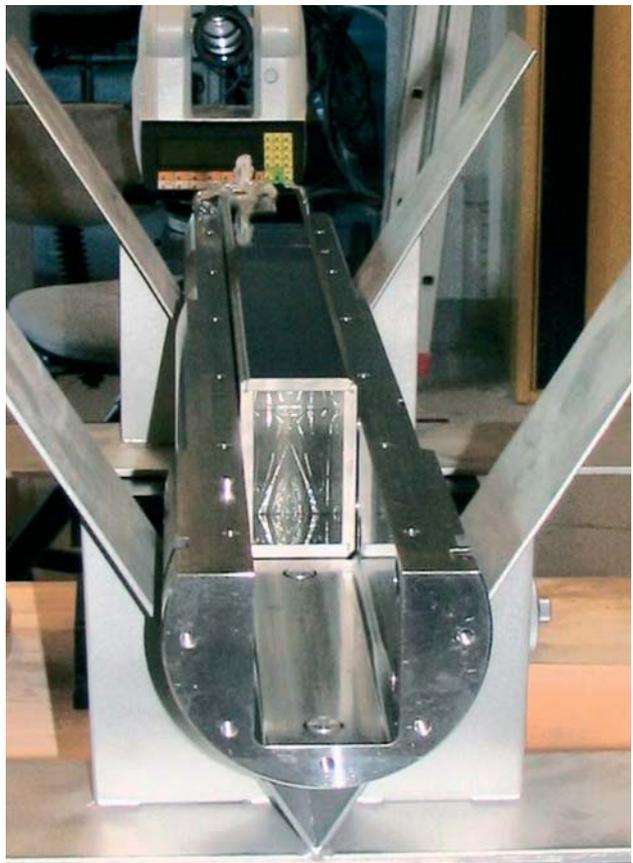
**Figure 5.** Alignment of the mirrors in the collimator
