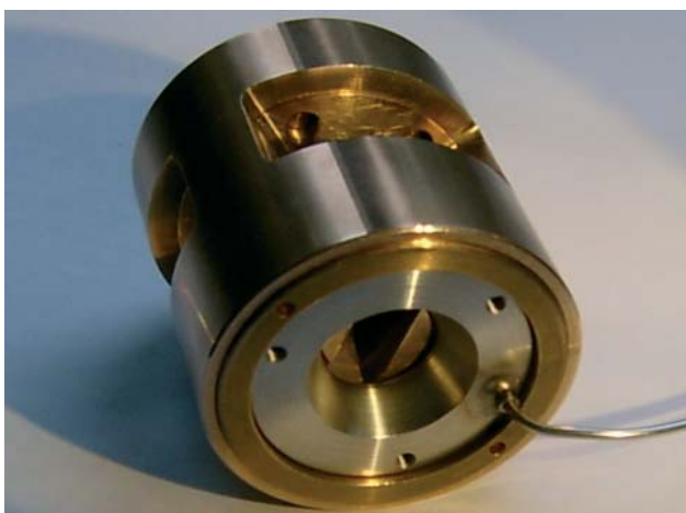
Figure 1. The “hybrid” cell; the latest generation of high pressure cell compatible with X-rays and neutrons.
