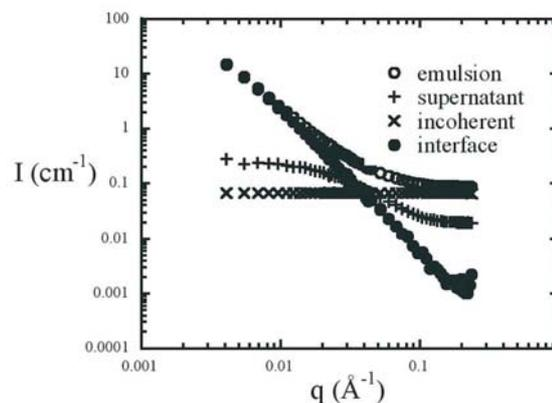
**Figure 1.** Specific treatment of emulsion measurements in the two liquid phase matching contrast condition to extracted the interface scattering signal after subtraction of the contributions of both incoherent scattering and asphaltene bulk scattering.
