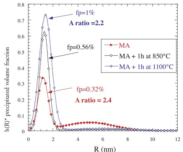
Figure 2 :  $Y_2O_3$  size distribution evolution under thermal treatment.
