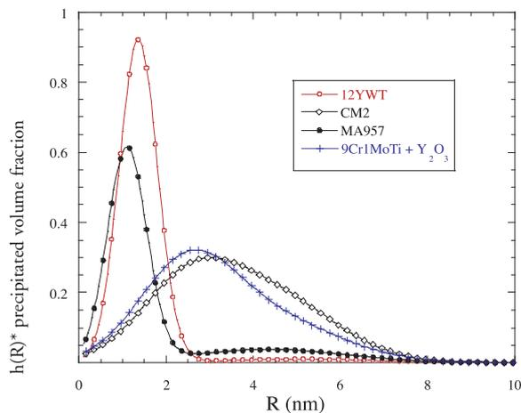
Figure 1 :  $Y_2O_3$  clusters size distribution in consolidated ODS alloys.
