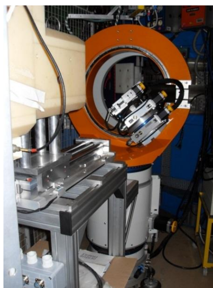
Figure 41: 6T1 sample support with translations x, y, z incorporated into Euler cradle.
