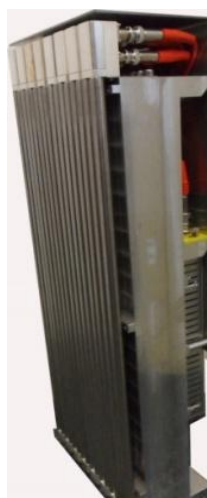
Figure 30: a detection module of 7C2: 16 tubes (paired at bottom) plus their electronics.
