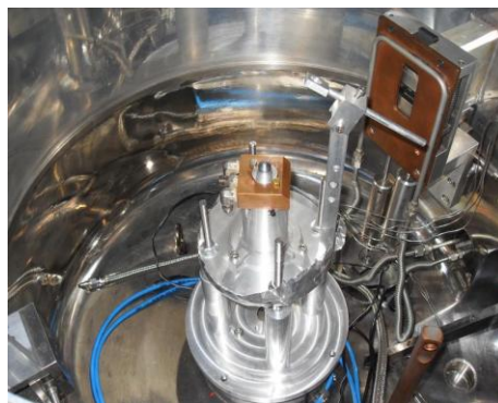
Figure 32: the gas levitation nozzle in the 7C2 vacuum chamber.
