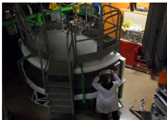
Figure 31: assembling the detector of the new 7C2 (the scattering angle width is around 135°).
