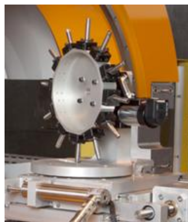
Figure 42 Automatic sample changer with 12 positions for texture measurements on super 6T1 at LLB.
