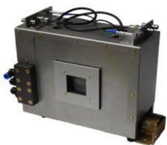
Figure 20 The new RF coils used for neutron-resonance spin-echo spectrometry.
