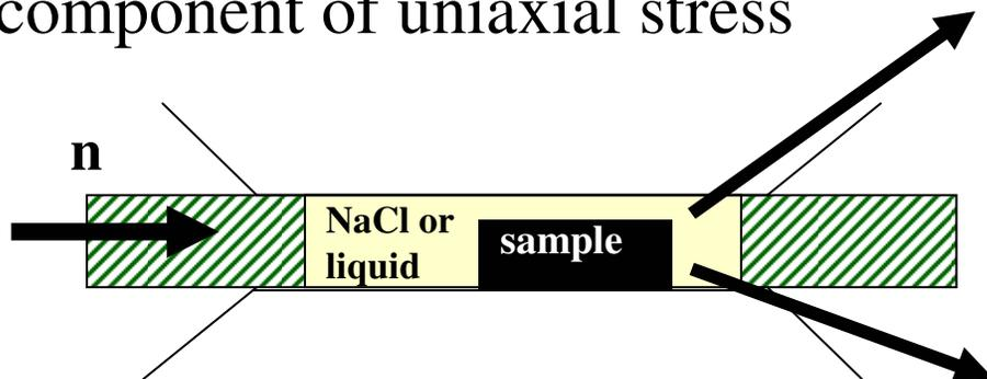
*Measurement of anisotropic stress by scanning the diffraction cone from NaCl*
