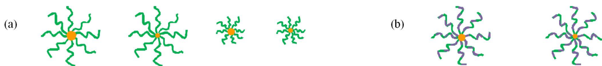
Figure 2.14: Thermoresponsive gold nanoparticles synthesized by "Grafting-to" via the one-step technique:(a)Au-PNIPAM ( M_w = 7861 - 29650 \text{ g.mol}^{-1} and D = 4.5 - 8.0 nm) and (b) Au-PNIPAM-co-NPAM (NIPAM:NPAM = 2.4:1 to 1:1 and D = 2.9 - 5.3 nm).
