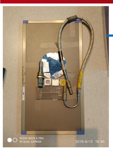
Image Plate mounted behind a lead shield
