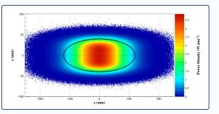
Beam density on target. Maximum density ;  $500 \text{ W cm}^{-2}$ .
