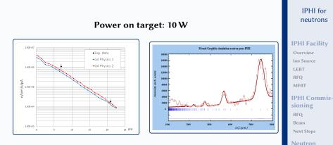
Gold disks measurements inside the moderator (dots) GEANT4 Monte Carlo simulations (lines)
