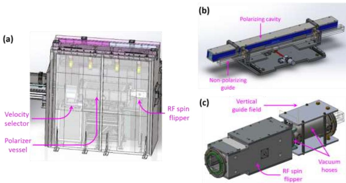
**Fig. 4 – (a) Casemate of the SAM instrument. (b) Polarizer/guide translation table. (c) RF spin flipper and subsequent guide field. Both are installed around the vacuum hoses connecting the polarizer and collimator vessels.**
