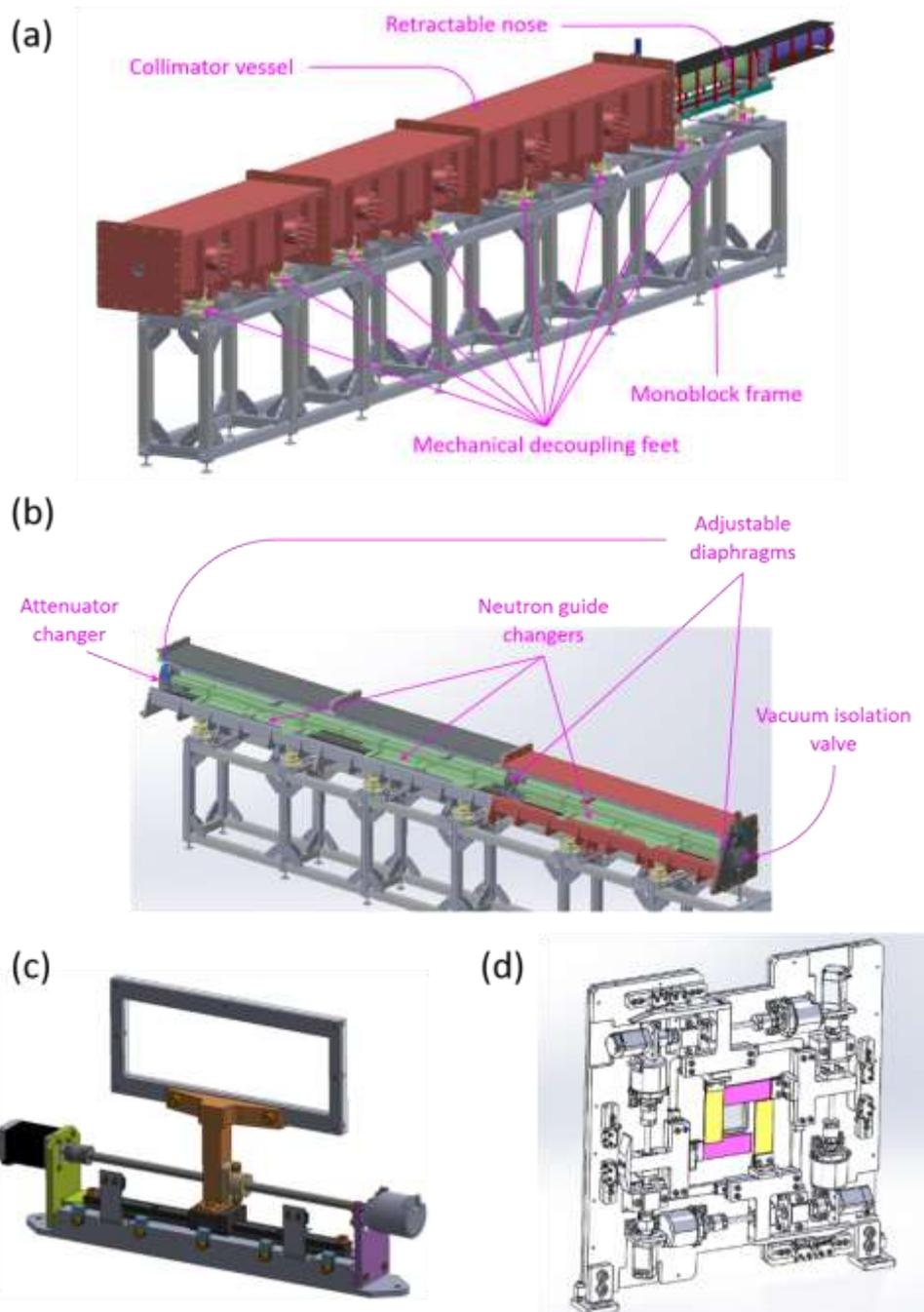
**Fig. 5 – (a,b) Collimator of the SAM instrument. (c) Linear attenuator changer. (d) Adjustable diaphragm with 4 independent blades.**
