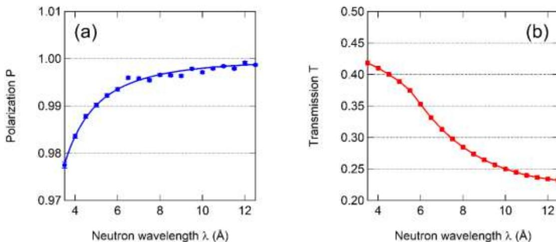
**Fig. 8 – Simulated wavelength-dependence of the beam polarization (a) and transmission w.r.t. incoming unpolarised beam (b).**
