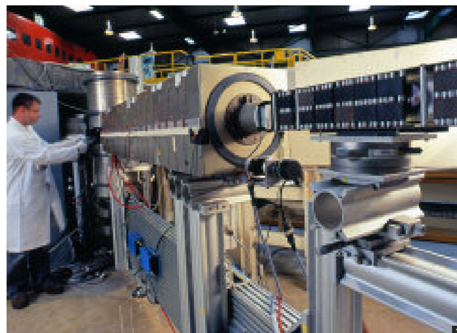
1. Installing a sample on a spin echo spectrometer for measuring slow molecule movement.
