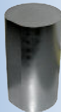
Silicon ingot irradiated at ORPHÉE. Their diameter can reach 15cm.
