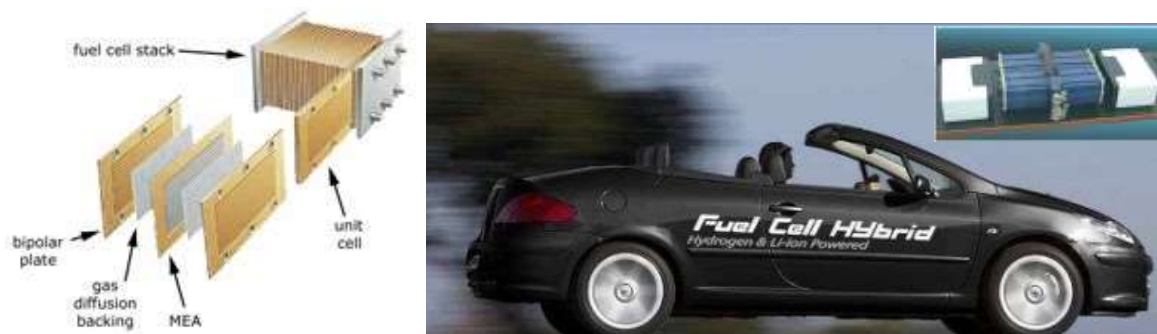
Figure 2. (a) Schematic drawing of a PEMFC stack and single cell. (b) Picture of an Hybrid Fuel Cell car integrating a PEMFC stack developed at CEA (inserted picture)
