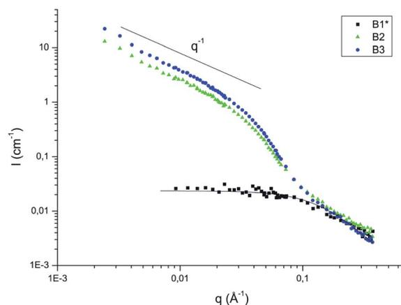
**Fig. 7** SANS intensity ( $I$ ) versus scattering vector ( $q$ ) for monomer **B1\*** and oligomers **B2** and **B3** solutions in  $CD_3OD$  at  $10\text{ g L}^{-1}$  and  $25\text{ }^\circ\text{C}$ .
