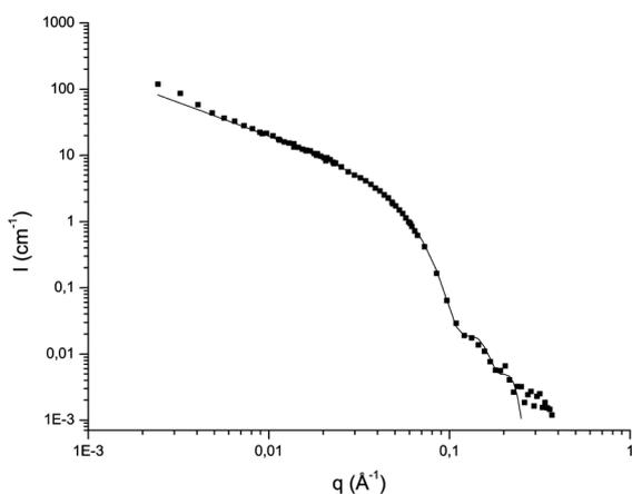
**Fig. 6** SANS intensity ( $I$ ) versus scattering vector ( $q$ ) for monomer **B1\*** solution in  $D_2O$  at  $10\text{ g L}^{-1}$  and  $25\text{ }^\circ\text{C}$ . The plain curve is a fit according to a model for two populations of long rigid filaments with a circular cross-section (respective cross-section diameters: 5.6 and 7.5 nm).
