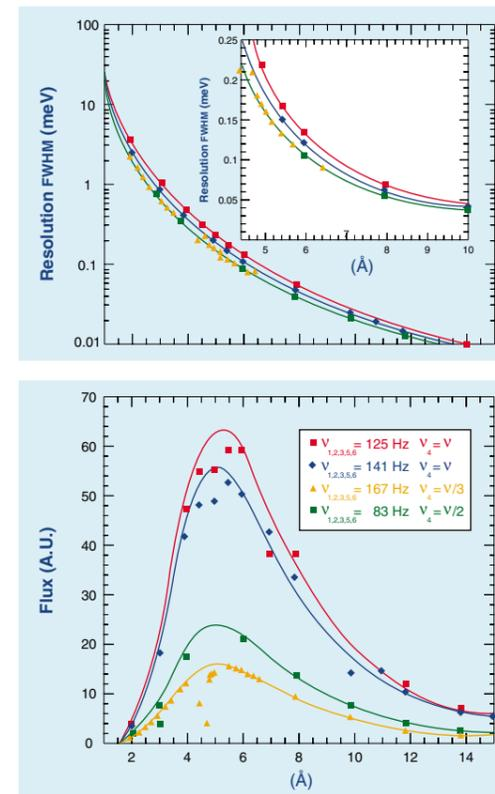
Fig. 1 : Examples of some achievable instrumental conditions on Mibémol as function of neutron incident wavelength.
