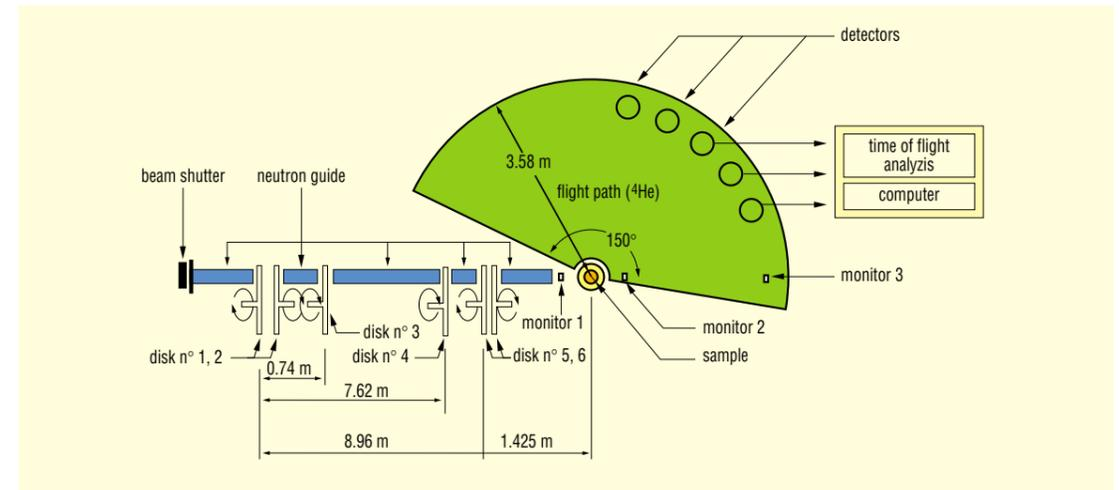
General layout of the time-of-flight spectrometer G 6-2.
