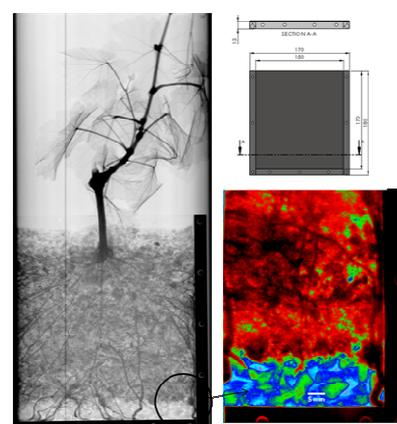
Figure 4: Neutron images of a grapevine herbaceous cutting cultivated by the AgroEcology team (Dijon) in an aluminium flat container (LLB design, Helary A.). The left « black and white » image has been performed with an image plate detector (neutronography station G4.5) and the right color one comes from the IMAGINE station (40 s of exposure), with
