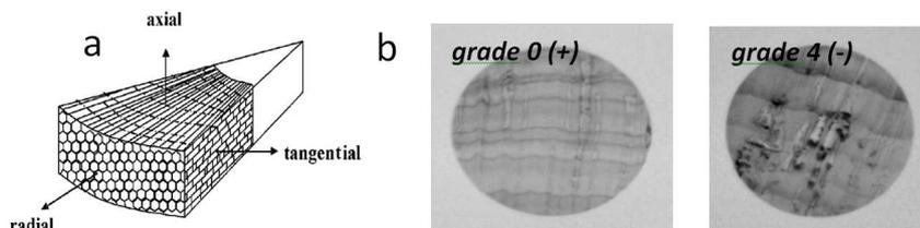
Figure 2: a- three dimensional structure of the cork from Silva et al. 2005 / b: Neutron radiographies of two slides of different qualities cork stoppers (IMAGINE instrument, 120 s exposure, 100  $\mu$ m scintillator)
