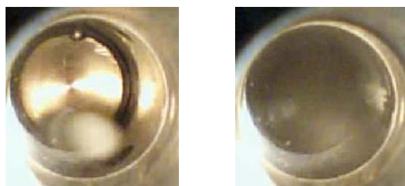
Fig. 2: Cloud point observation. Left: the polymer is soluble and light reflexes are transmitted through the sample. Right: the system is below the cloud point and thus opaque.
