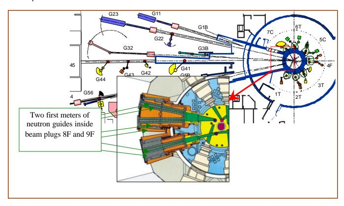
Figure. General layout of the guides elements within the 8F and 9F beam plugs.
