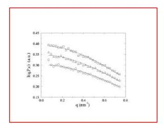
Scattering spectra I(q,P,c) of  $MbN_3$  at  $p^2H$  7, as a function of the wave-number transfer q. The measurements were performed at  $20^{\circ}C$ . The protein concentration at atmospheric pressure (0.1 MPa) was c(0.1) = 11.7 mg cm<sup>-3</sup> and the pressures, P, were: 54 (?), 154 (?), and 302 Mpa (?). Fits of the Guinier approximation to the data are shown as full lines.
