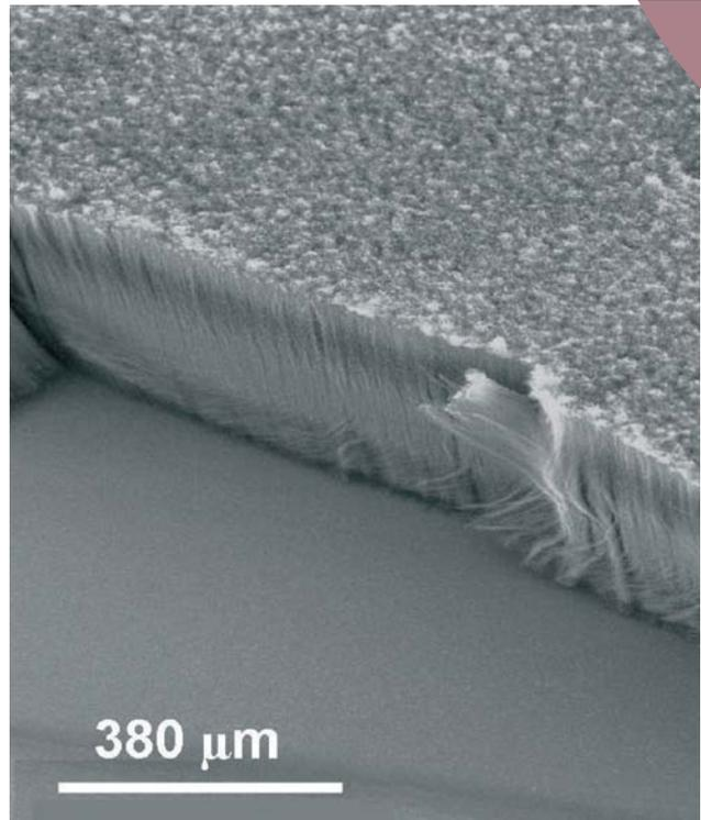
**Figure 4** (from Ref.3). Scanning Electron Microscopy image of aligned carbon nanotubes (a-CNT) synthesized on silicon substrates by aerosol-assisted catalytic chemical vapour deposition from toluene/ferrocene aerosol. The a-CNT obtained are multiwalled (J. M. Pinault *et al.*, Nano Lett., 5, 12, 2394-2398 (2005).
