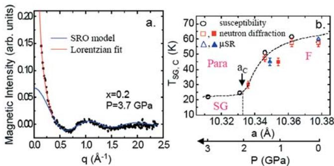
**Figure 3.** a. Magnetic intensity for  $x=0.2$  sample at 1.4 K and 3.7 GPa. Lines are fits using SRO model and Lorentzian fit respectively. b. Phase diagram for  $(\text{Tb}_{1-x}\text{La}_x)_2\text{Mo}_2\text{O}_7$  in the threshold region: ambient pressure (open symbols) and under pressure (full symbols).
