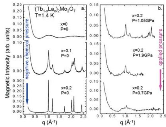
**Figure 1.** Magnetic intensity of  $(\text{Tb}_{1-x}\text{La}_x)_2\text{Mo}_2\text{O}_7$  at 1.4 K versus the scattering vector  $q=4\pi\sin\theta/\lambda$ . The neutron wavelength is  $\lambda=4.741 \text{ \AA}$ . A spectrum in the paramagnetic phase (70 K) was subtracted and the magnetic intensity was scaled to the (222) nuclear peak intensity.
