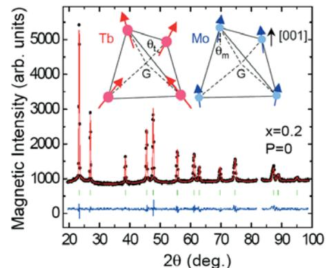
**Figure 2.** Magnetic intensity for  $x=0.2$  at 1.5 K versus the scattering angle  $2q$ ,  $\lambda=2.426 \text{ \AA}$ . A 70 K spectrum was subtracted. Solid lines show the best refinement and the difference spectrum (bottom). In inset: magnetic structure of the Tb- and Mo- tetrahedra.
