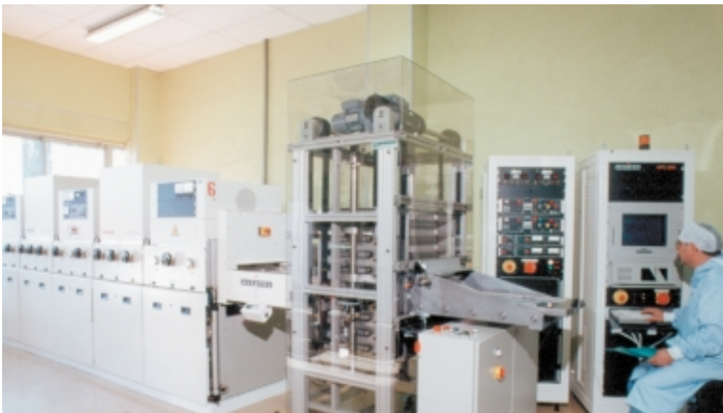
Guide coating by sputtering. General view of the machine used for producing supermirrors coating (CILAS photography).
