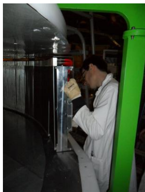
Carefully installing our 16 invaluable detection moduli with 30b\ ^3\text{He} PSD tubes
